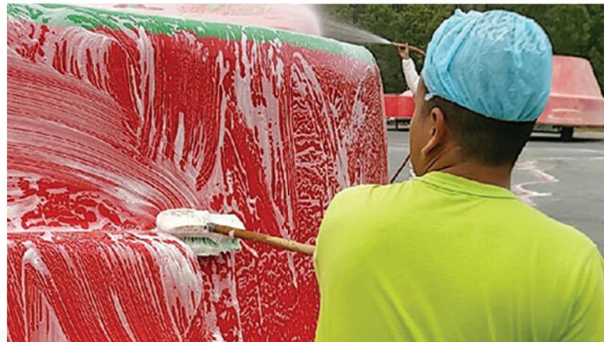
The mold is cleaned and prepared to build your pool.
